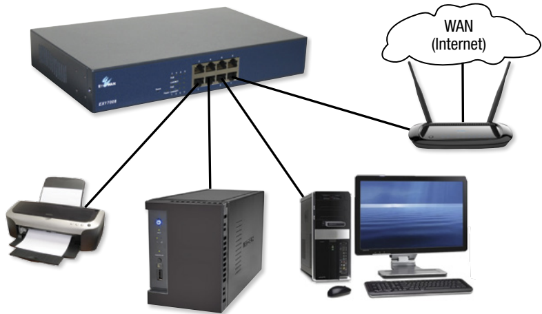
In the diagram above you can see that Ethernet switches are used for sharing resources such as printers, networked file servers and router connections to the Internet or Wide Area Network (WAN).
